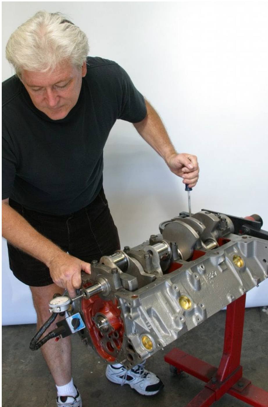
Crankshaft endplay should be .004-.008-inch maximum. (Image/Jim Smart)
