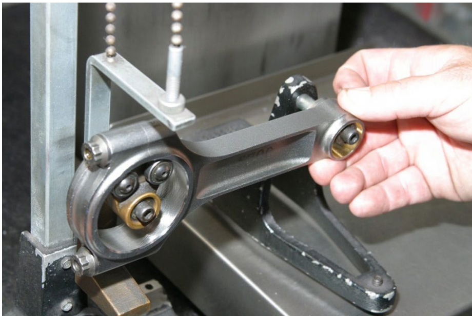
Although our stroker kit was pre-balanced, L&R Engines checked dynamic balance a second time for added assurance. (Image/Jim Smart)
